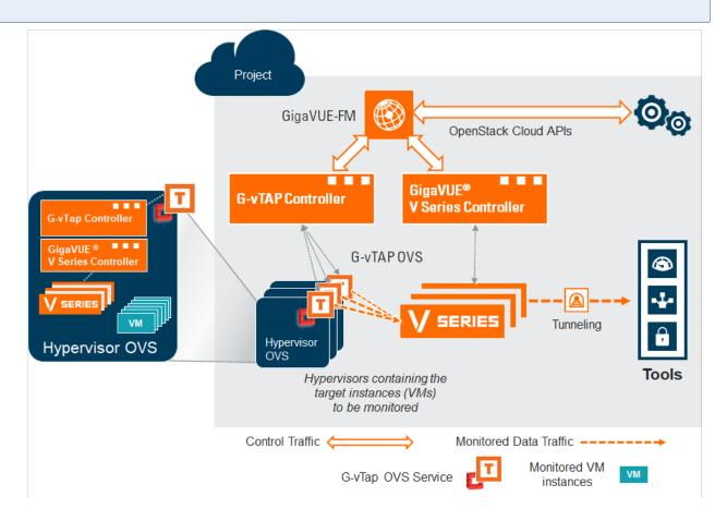
**Figure 2** GigaVUE Cloud Suite Cloud Components for OpenStack using OVS Mirroring or OVS Mirroring + DPDK
